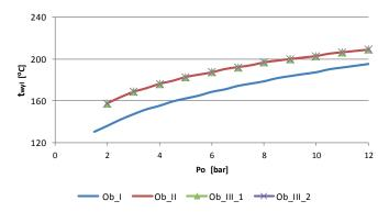
Fig. 8 Temperature of exhaust gas from waste heat boiler in function of live steam pressure as well as the feed-water temperature in degasifier, todg=150 °C, for 9K98MC engine
