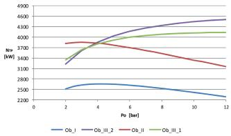
Fig. 5 Steam turbine power output in function of live steam pressure as well as the feed-water temperature in degasifier, todg=150 °C, for 9RTA96C engine
