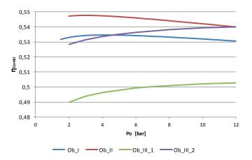
Fig. 7 Efficiency of the combined systems in function of live steam temperature as well as feed-water temperature in degasifier, todg=150  $^{\circ}$ C, for 9RTA96C engine
