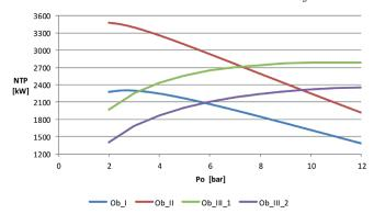
Fig. 4 Steam turbine power output in function of live steam pressure as well as the feed-water temperature in degasifier todg=150  $^{\circ}$ C, for 9K98MC engine
