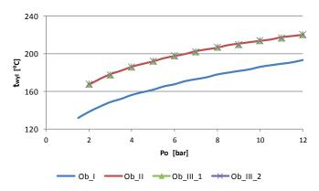
Fig. 9 Temperature of exhaust gas from waste heat boiler in function of live steam pressure as well as the feed-water temperature in degasifier, todg=150 °C, for 9RTA96C engine
