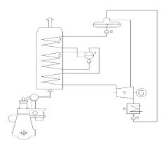
Fig. 1. Variant of a power system with one-pressure cycle Designations: 1. Steam superheater, 2. Boiler proper, 3. Economizer, 4. Boiler drum, 5. Steam turbine, 6. Condenser, 7. Degasifier, 8. Main feed-water pump, 9. Condenser pump.
