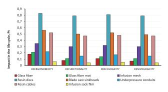
Fig.5. Life-cycle impact of 1 kg amount of man-made and natural materials and elements being post-service waste from the rotor blade of the wind electric power plant, related to various kinds of its destructiveness (acc. these authors' original work)
