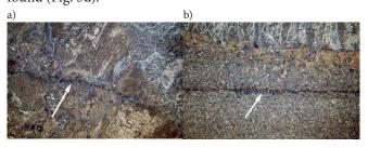
Fig. 6. Cracks occurred in the HAZ of the specimens: a) W1, magn. x 200; b) W2, magn. x 100
