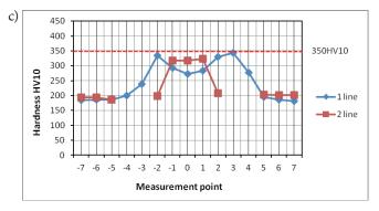
Fig. 9. Distribution of HV10 hardness values along the measurement lines 1 and 2 for the welded joints of the pipes without insulation coating:
