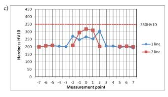
Fig. 8. Distribution of HV10 hardness values along the measurement lines 1 and 2 for the welded joints of the pipes with insulation coating: a) C1, b) C2, c) C3
