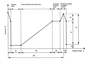
Figure 5. Theoretical pressure time-history in gear pump during full gear rotation
