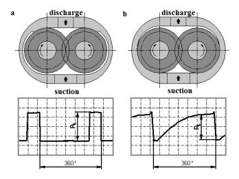
Figure 4. Schematic of circumferential sealing of gears and graph of circumferential pressure distribution measured in the tooth space: a - discharge side. b - suction side
