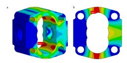
Figure 9. Location of measuring points of the maximum stress and displacement in the pump body
