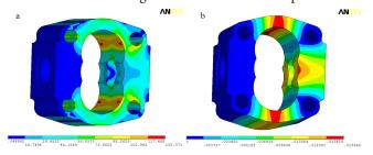
Figure 7. Distribution of stress(a) and displacement (b) in micropump body – initial position of bushings
