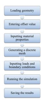
Figure 3. Algorithm of micropump body stress calculations
