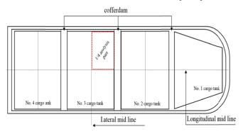
Fig. 1. Tank arrangements of KC-1 LNG carrier
