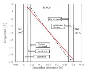
Fig. 5. Temperature profile of KC-1 insulation (black dot: results of  $\mathbf{q}_{ins}$ , red solid: results of  $\mathbf{q}_{H-PUF}$ )
