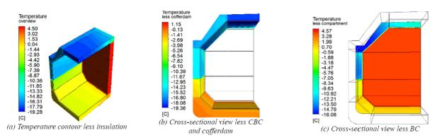
Fig. 8. Temperature contour of base tank case, USCG-2, for USCG condition
