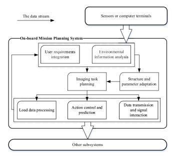
Fig. 2. Structure of proposed on-board mission planning system
