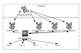
Fig. 1. Earth observation system (EOS) of traditional imaging satellite
