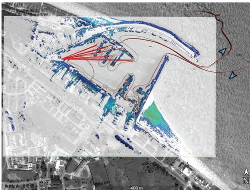
Fig. 9. Trajectory of the scanner movement imposed on Google Earth™ for the port: raw red colour and aligned – green, with the designation of exit and entrance to the port
