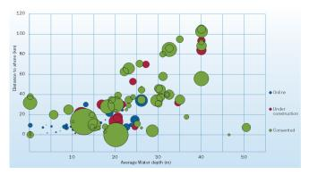
Fig. 4. Development trends in offshore wind power industry in function of distance to shore and water depth in site of new installations [9]
