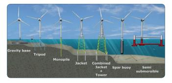
Fig. 1. Various solutions of anchoring the offshore wind power electric plants, depending on water depth [3]
