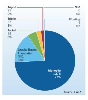
Fig. 2. Relative amount of power installed in 2012, depending on an applied manner of the anchoring of foundation of offshore wind power electric plant [9]
