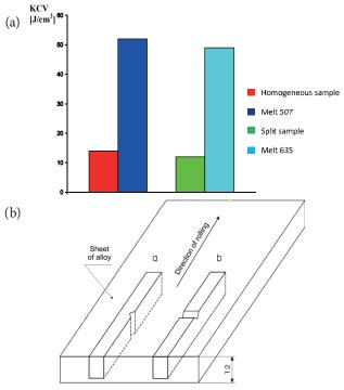
*Fig.2. a)- Average impact resistance of homogeneous and split samples* (*h*1=*h*2=0,5*h*) of 7020M alloy. Samples taken from melts 507 and 635. *b)- Method of cutting samples from a sheet of the examined alloy 7020M*
