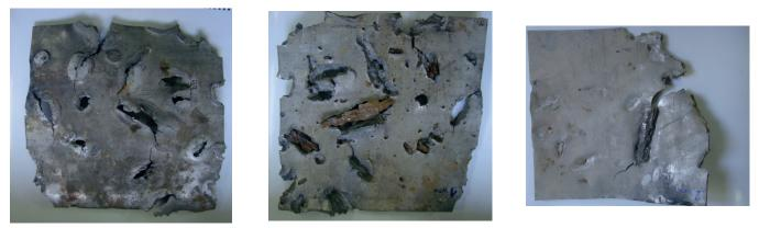
Fig.9. Effects of 7020M alloy sheet perforation (dimensions 300x3000): a) homogeneous g = 12 mm b) split (w-inner, z –outer from the source of explosion, total thickness g = 2x6 mm) after detonation of high explosive shell of OF412 type and calibre 100 mm with the contents of 1,4 kg of TNT, taking place at a distance of 0,6 m.
