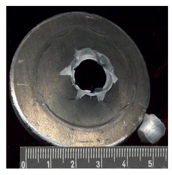
Fig.8a. Effects of firing the LPS shell with steel core and the energy of 3 kJ to 7020M alloy from the dis-tance of 2 m - unprotected sample
