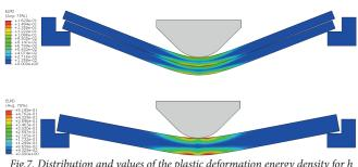
Fig.7. Distribution and values of the plastic deformation energy density for h = 0,6 m (J/m3)
