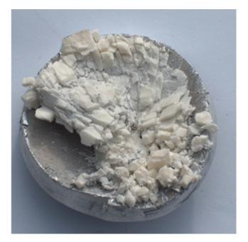
Fig.8b. Effects of firing the LPS shell with steel core and the energy of 3 kJ to 7020M alloy from the dis-tance of 2 m - sample protected with ceramic  $Al_2O_3$  of g = 6 mm
