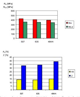
Fig.1. Static mechanical properties of 7020M and 7020 alloys (melts 507 and 635) and 7020 alloy (melt 484/4), samples cut from sheets of g = 12 mm, according to the direction of rolling
