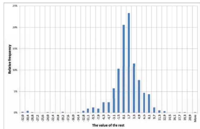
Fig. 7. Distribution of residuals ( $NO_x - NO_x$ ) for the neural model  $NO_x$ .  $NO_x = f(M_o, n)$  – experimentally measured content of  $NO_x$  in the exhaust gas,  $NO_{xs}$  – neural network response obtained for the set values of ( $M_o, n$ )
