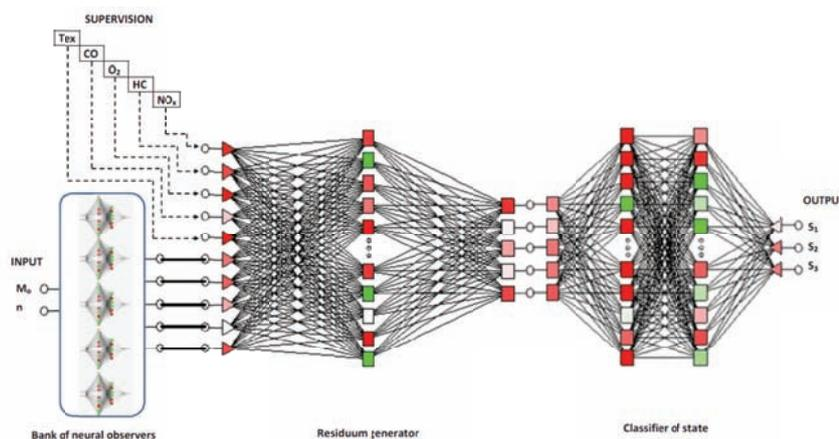
Fig. 3. Scheme of neural damage detection system.  $M_o$  – engine torque,  $n$  – engine rotational speed,  $T_{ex}$  – exhaust gas temperature,  $CO$  – content of carbon monoxide in the exhaust gas,  $O_2$  – content of oxide in the exhaust gas,  $HC$  – content of aromatic hydrocarbons in the exhaust gas,  $NO_x$  – content of nitrogen oxides in the exhaust gas
