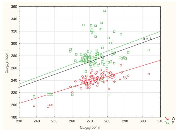
Fig. 2. Concentration of hydrocarbons HC for unsteady state at  $n = 1100$  rpm and load change from  $M_o = 30$  Nm to  $M_e = 50$  Nm: P - delayed injection advance angle, W - advanced injection advance angle, CHC (N, W, P) - HC concentration for (N) nominal, (W) advanced, and (P) delayed injection advance angle
