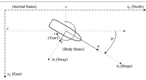
**Fig. 1.** Definition of the adopted coordinate systems: inertial frame (earth-fixed frame)  $x_e y_e z_e$ and body frame (body fixed frame)  $x_b y_b z_b$  connected with the moving ship
