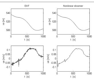
Fig. 5. Experimental data: measured position with estimate and estimated velocity u in surge. Left-hand column – extended Kalman filter, right-hand column – nonlinear observer
