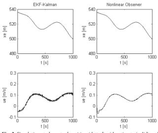
Fig. 2. Simulation study: actual position (dotted) with estimate (solid) and actual velocity u in surge (dotted) and estimate (solid)
