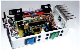
Fig. 10. Electronic elements for tunnel thrusters drive
