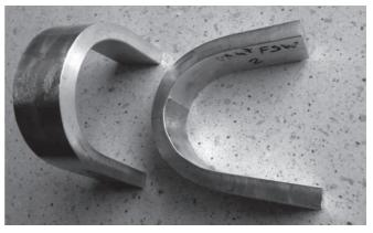
Fig. 2. A view of FSW method-welded specimens after bending tests
