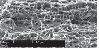
Fig. 3. Fracture of AW-7020 alloy joint welded by FSW, achieved during SSR test
