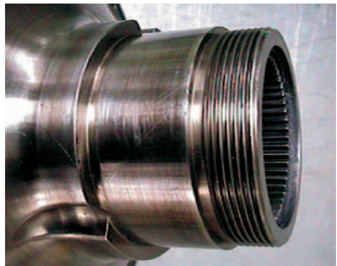
Fig. 2. Central bearing journal, connection between two shaft parts (turbine shaft, compressor shaft)
