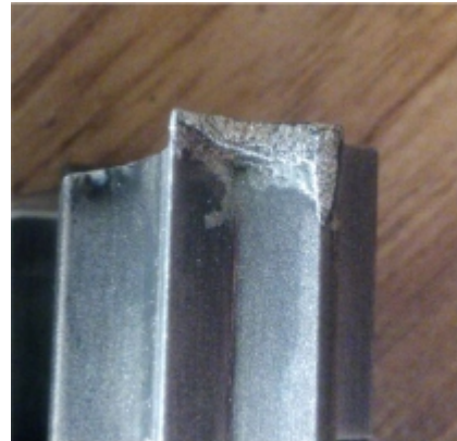
Fig.6. Repaired area before machining.
