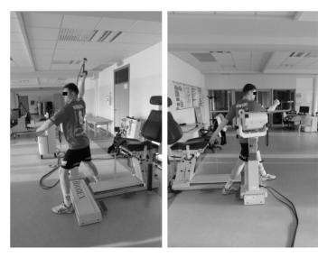
Figure 2. Measurement of the net torque of the muscles of the kinematic chain going from the trail leg to the hand of the dominant limb. Left: start position. Right: end position
