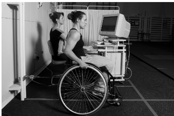
Figure 3. Propelling force measurement with hands placed on the middle of the pushrim (FP2)
