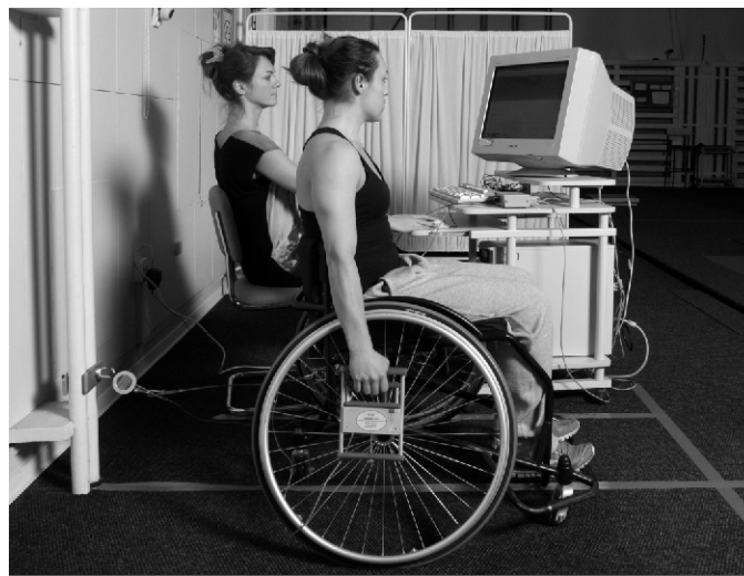
Figure 1. Grip strength measurement using a tensometric dynamometer
