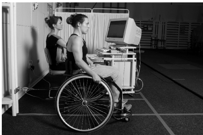
Figure 4. Propelling force measurement with hands placed on the front of the pushrim (FP3)
