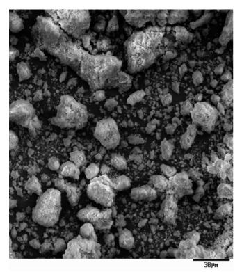
Figure 3. SEM microphotograph of chromium(III) silicate, sample 2
