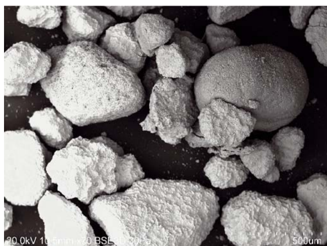
Figure 8. The SEM image of fly ash (A, x200) and slag (B, x200) after Pb(II) adsorption
