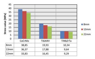
Figure 6. The influence of the sled's cross section radius and insert's thickness on the value of generated stress in the UHMWPE insert
