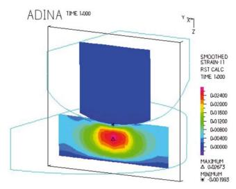
Figure 5. Material strain distribution occurring in sub-surfaces of spherical polyethylene insert cooperating with metal sled. Cross section of the model. Sled of cross section radius 27 mm. Load 1500 N
