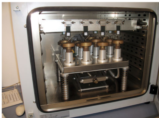
Figure 3. Evaluation of the shear strength of self-adhesive materials
