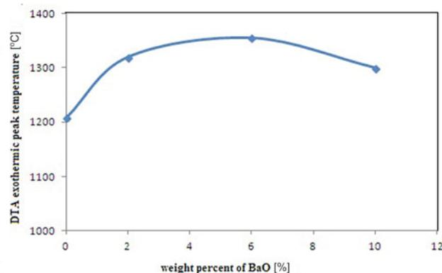
**Figure 1.** Relationship between the DTA exothermic peak temperature of the  $\gamma$ -to- $\alpha$  phase transition and weight percent of barium oxide
