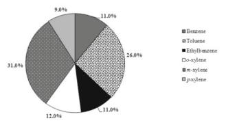
Figure 1. The average weight percentage of BTEX in petrol<sup>1</sup>
