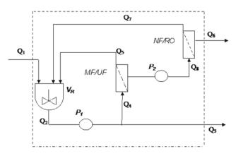
Figure 3. Schematic diagram of a bioreactor with two separation modules (VR – reactor volume, MF/UF – first step of filtration, NF/RO – second step of separation)
