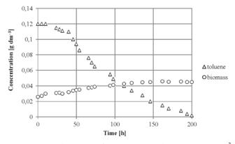
Figure 6. Batch process of toluene removal ( $c_{S,0} = 0.12 \text{ g dm}^{-3}$ , 24°C): ( $\Delta$ ) toluene concentration, (o) biomass concentration
