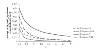
Figure 9. Average pollutant concentration in the merged outgoing (Q3 and Q6) streams as a function of  $\Psi$  and R<sub>s</sub> (based on Equation (14))
