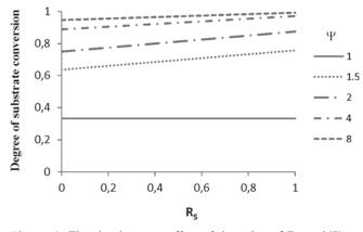
Figure 4. The simultaneous effect of the value of  $R_s$  and  $\Psi$  on the degree of substrate conversion (based on Equation (15))
