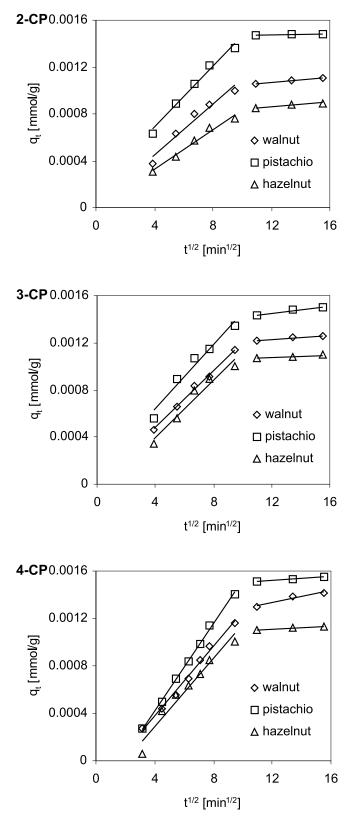
Figure 5. Intraparticle diffusion model for the sorption of 2-CP, 3-CP and 4-CP on nut shells
