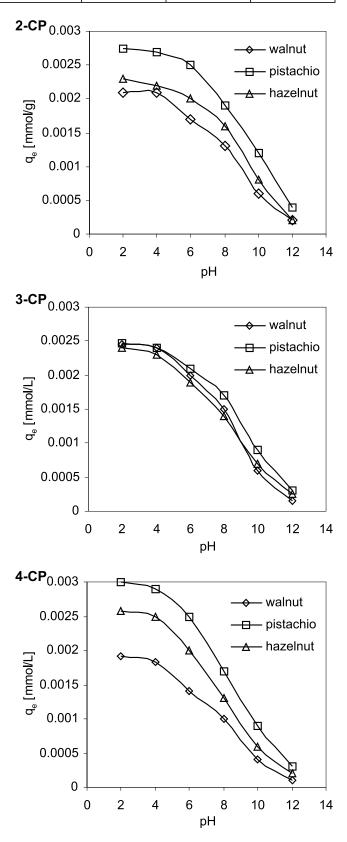
Figure 3. Effect of pH on the sorption amount of 2-CP, 3-CP and 4-CP on nut shells
