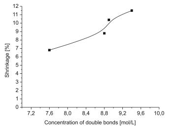
Figure 2. Shrinkage of dental composition containing multifunctional methacrylates versus concentration of double bonds in methacrylates
