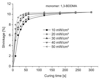
Figure 5. Shrinkage of dental filling containing monomer 1,3-BDDMA versus curing time and UV curing dose
