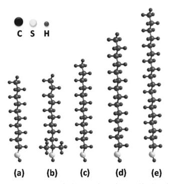
Figure 1. Structure of thiols used for surface modification of gold nanoparticles: 1-decanethiol (a), 1,1-dimethyldecanethiol (b), 1-dodecanethiol (c), 1-tetradecanethiol (d), 1-octadecanethiol (e)
