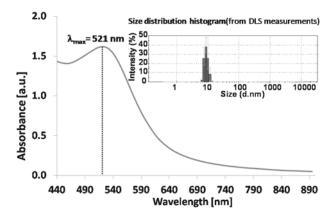
**Figure 2.** UV-Vis absorption spectrum and the size distribution histogram from DLS measurements (by intensity) of the aqueous AuNPs stabilized with mixture of citrate and tannic acid
