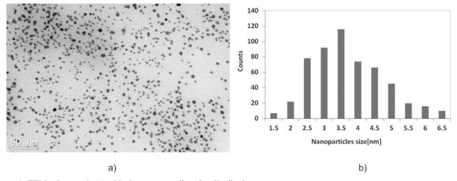
Figure 4. TEM micrograph (a) with the corresponding size distribution
