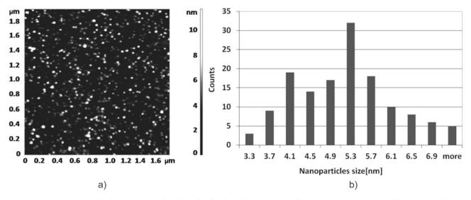
Figure 3. AFM image (a) with the corresponding size distribution histogram (b) of the aqueous AuNPs stabilized with mixture of citrate and tannic acid
