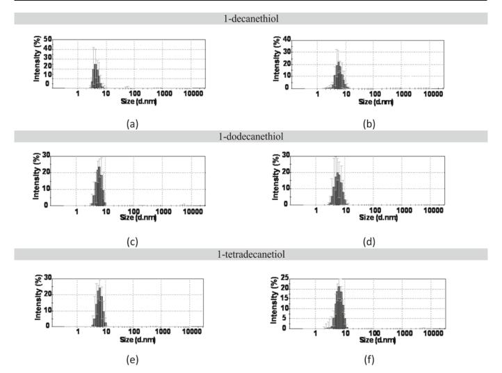
Figure 6. The size distribution histograms of the gold nanoparticles in toluene modified with 1-decanethiol, 1-dodecanethiol and 1-tetradecanethiol after the phase transfer process (a), (c), (e) and after 2 months (b), (d), (f)
