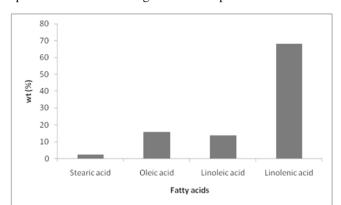
Figure 3. Fatty acid composition of linseed oil biodiesel
