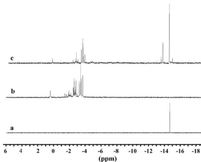
**Figure 4.**  $^{31}\text{P}$  NMR spectrum of: (a)  $\text{H}_3[\text{PW}_{12}\text{O}_{40}]\cdot\text{aq}$ , ca. 0.1 M; (b)  $\text{H}_3[\text{PMo}_9\text{V}_3\text{O}_{40}]\cdot\text{aq}$ , ca. 0.1 M; (c) mixture of the two solutions; the spectrum was recorded 20 nm after preparation of the solution (solvent  $\text{D}_2\text{O}/\text{H}_2\text{O}$  1/1,  $T = 297$  K)
