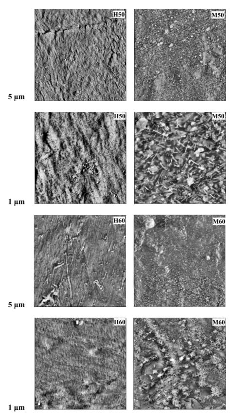
Figure 4. The AFM phase images of TPUs H50, H60, M50 and M60 at 5 and 1  $\mu m$  scan sizes
