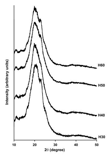
Figure 6. The XRD patterns of the HDI-based TPUs
