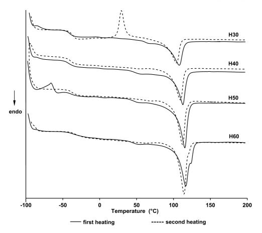
Figure 2. The DSC curves of the HDI-based TPUs
