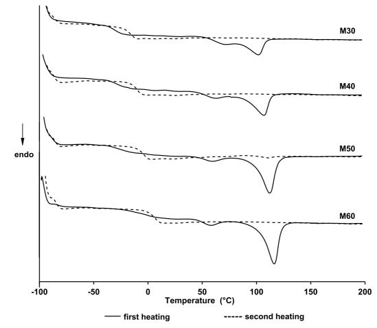
Figure 3. The DSC curves of the MDI-based TPUs
