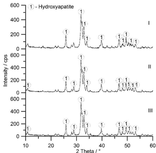
**Figure 4.** The diffractogram of the ash from mixtures I, II and III calcined at 600°C
