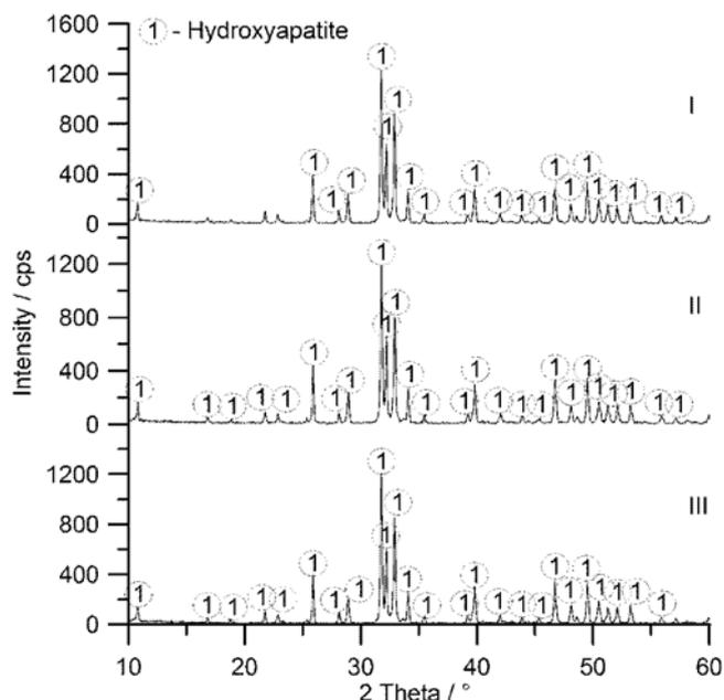
Figure 5. The diffractogram of the ash from mixtures I,II and III calcined at 800°C
