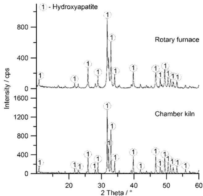
Figure 7. The diffractogram of the ash from mixture III calcined at 900°C in the rotary furnace
