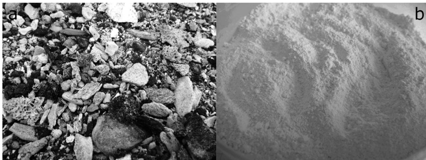
Figure 8. Ash: a – calcining of the mixture of bone waste in the rotary furnace at the temperature of 900°C, b – after comminution and second roasting
