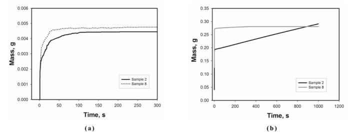
Figure 6. Comparison of (a) sedimentation profiles and (b) wettability in water systems obtained for samples 2 and 8
