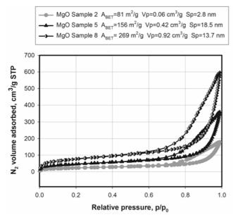
Figure 4.  $N_2$  adsorption/desorption isotherms for samples 2, 5, 8
