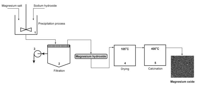
1 - reactor 2 - pressure filter 3 - vacuum pomp 4 - stationary drier 5 - oven
