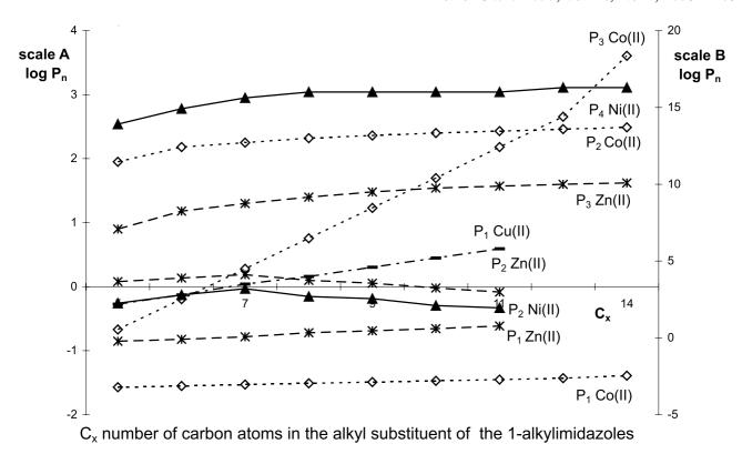
Figure 3. The influence of the alkyl chain length on the partition ratios  $(P_n)$  of Co(II), Ni(II), Cu(II), and Zn(II) complexes with 1-alkylimidazoles for methylene chloride [scale B – for  $log P_3$  of Co(II) – 1-alkylimidazole complexes]
