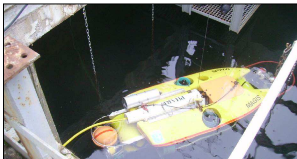
Fig. 2. Underwater vehicle MAGiS undergoing tests conducted by the Scientific Association ABYSAL in the Technological Pool of the Faculty.
