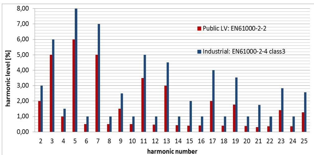
Fig. 2. Minimum requirements for harmonic immunity – compatibility levels
