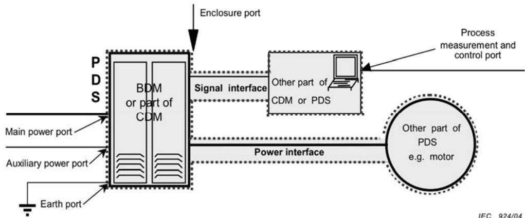
Fig. 1. Internal interfaces of the PDS and examples of ports according to standard [1]
