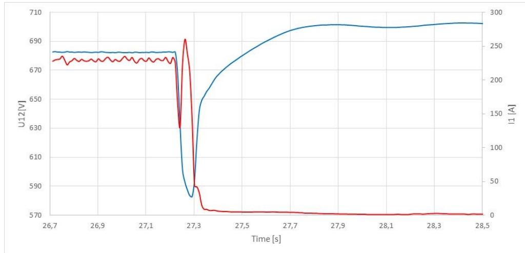
Fig. 3. Waveform of root-mean-square current and voltage at the terminals of the converter point of common coupling during a dip
