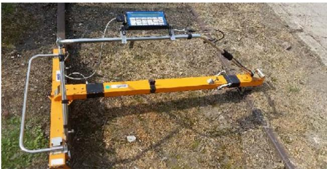
Fig. 1. The measuring device TEC-1535 N3. Own study
