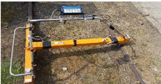
Fig. 1. The measuring device TEC-1535 N3. Own study
