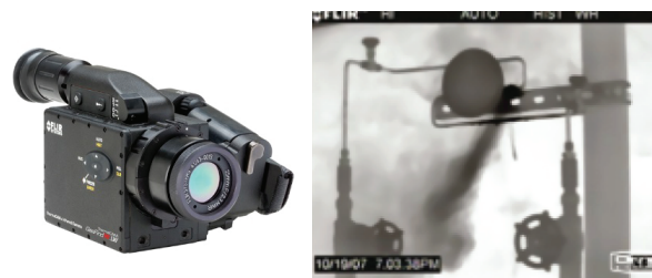
Figure 5. The GasFindIR camera showing the leakage of methane in the transmission installation.
