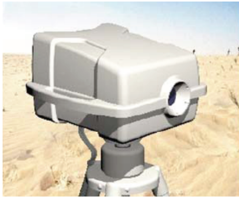
Figure 9. The AIRIS WAD contamination detection system [Marinelli et al. 2005].
