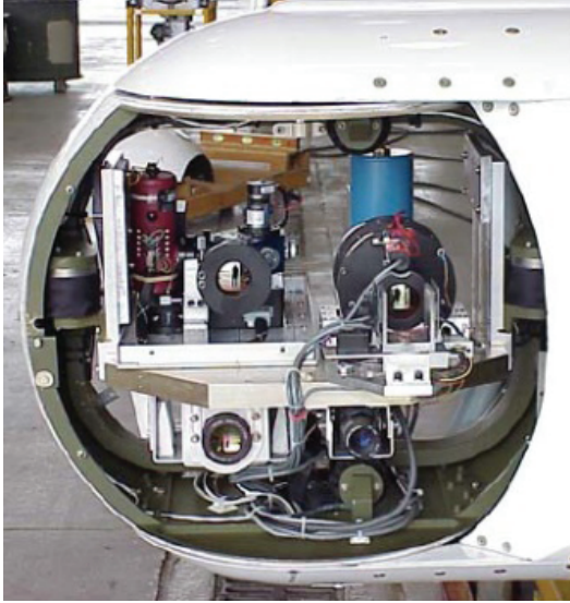
Figure 7. A FAT BOY device with the AIRIS-LW system mounted on a UH helicopter.
