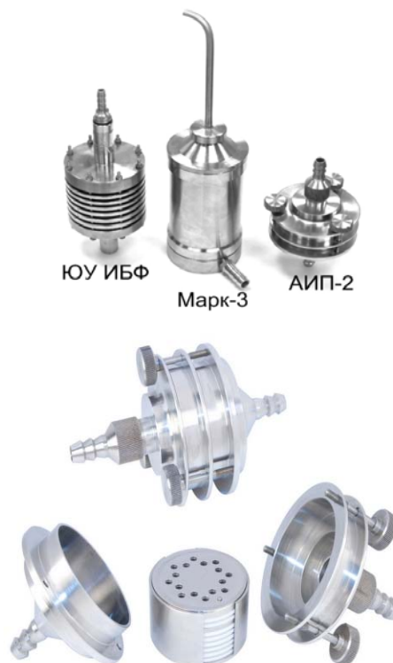
Fig. 4. The external and internal views of the AIP-2 cascade impactor.
