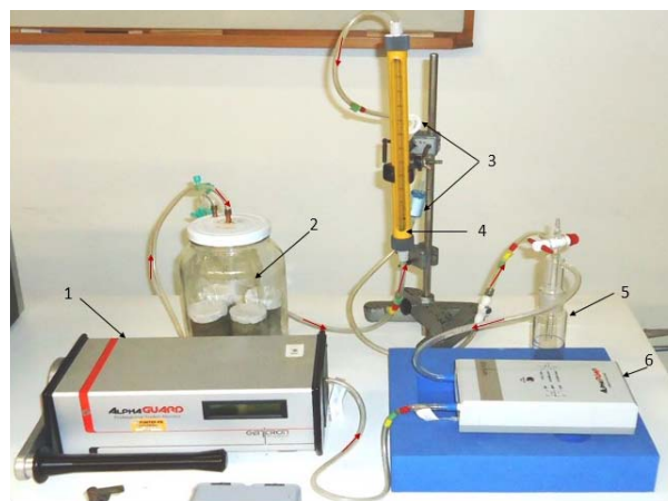
Fig. 3. Measurement of radon concentrations with AlphaGuard detector. 1 – AlphaGuard detector, 2 – samples within glass jar, 3 – filters, 4 – rotameter, 5 – glass container, 6 – air pump (AlphaPump).
