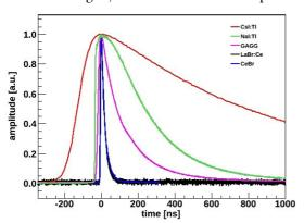
Fig. 2. Pulse shapes obtained from the tested scintillators.
