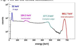
**Fig. 3.** Energy spectrum of 661.7 keV  $\gamma$ -ray line from a  $^{137}$ Cs source measured with the LaBr<sub>3</sub>:Ce scintillator.
