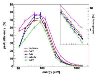
**Fig. 6.** Full energy peak detection efficiency measured for  $\gamma$ -rays with energies from 22.1 keV to 1408 keV. In the inset, the dependence for higher energies is shown in a double logarithmic scale. Lines are a guide for the eye.
