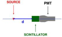
**Fig. 1.** Schematic of the experimental setup used in the described measurements, d – distance between the γ-ray source position and the front surface of the scintillator.
