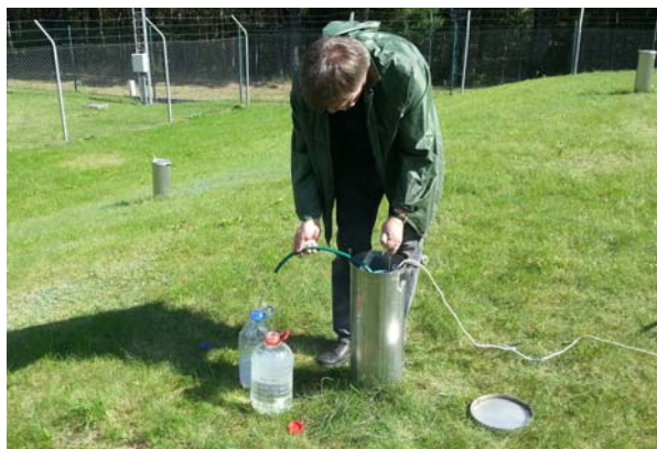
Fig. 2. Groundwater sampling from monitoring well no. 42. Monitoring wells no. 4, 5 and 41 are well seen in the picture.
