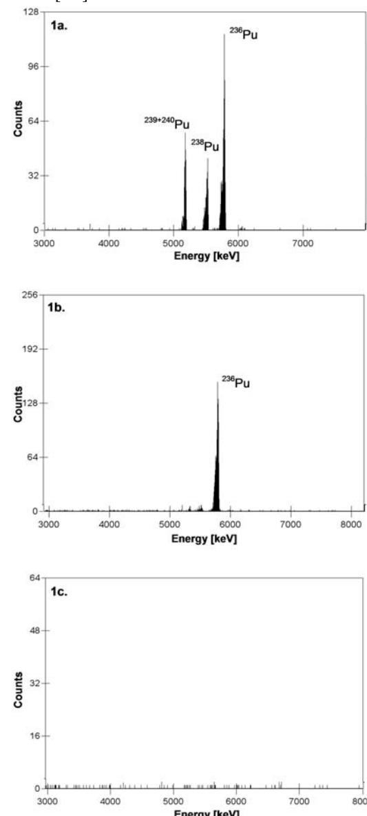
**Fig. 1.** Alpha spectra of a) urine sample with plutonium isotopes (<sup>236</sup>Pu, <sup>238</sup>Pu, <sup>239+240</sup>Pu), b) urine sample with tracer (<sup>236</sup>Pu), c) blank sample.
