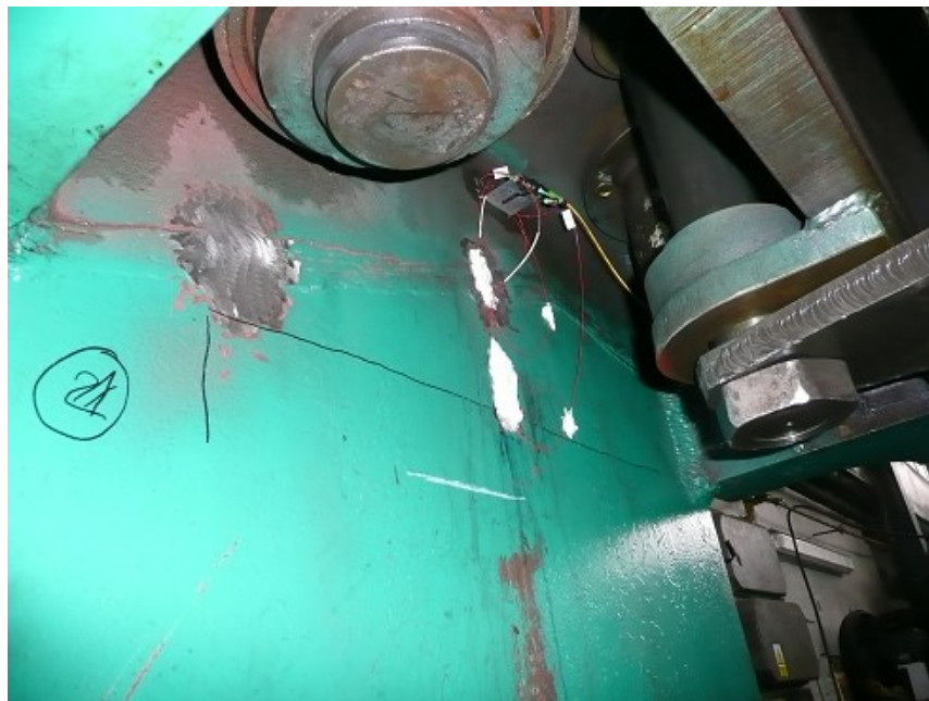
Fig. 3. Location for the strain sensors
