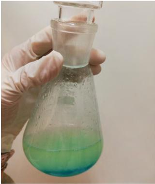
**Figure 3.** Over-titrated sample
