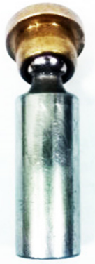
Fig.5.b) Piston failure of loose slipper.
