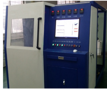
Fig.4.a) Hydraulic Pump Full Life Test Platform.
