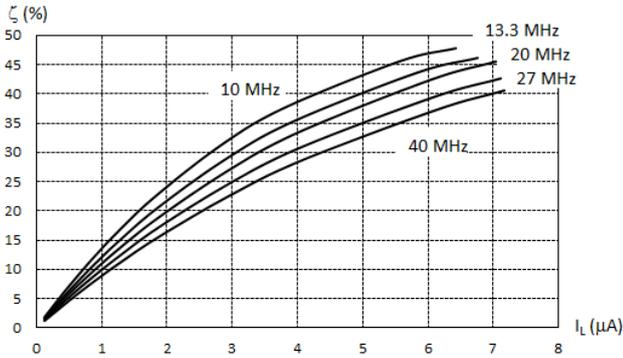
Fig.5. Efficiency as a function of  $I_L$  for  $N=6$ .
