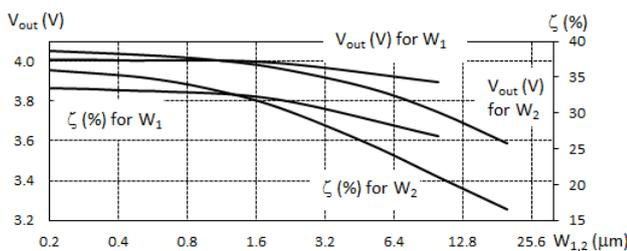
Fig.10. Option 4, 5: Efficiency and output voltage as functions of  $W_{1,2}$ .
