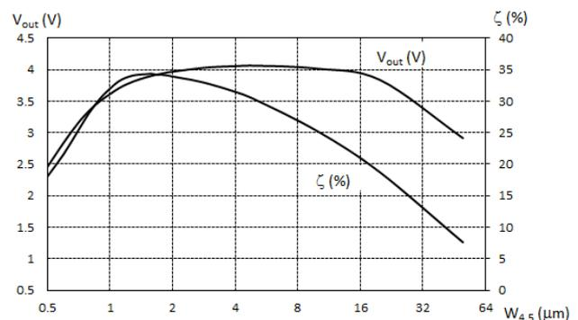
Fig.7. Option 1: Efficiency and output voltage as functions of  $W_{4,5}$ .
