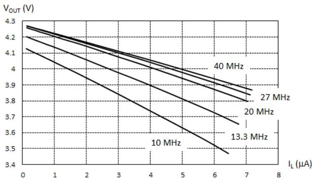
Fig.6. Output voltage as a function of  $I_L$  for  $N=6$ .
