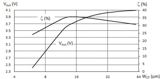
Fig.11. Option 6: Efficiency and output voltage as functions of  $W_{CT}$ .
