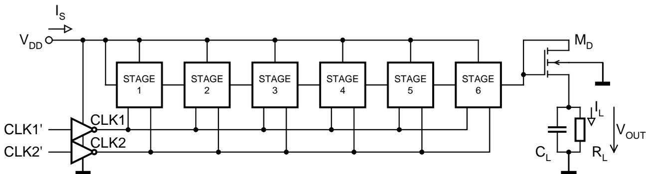
Fig.4. Simplified schematic diagram of the simulated charge pump for  $N=6$ .
