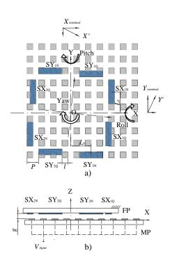
Fig.1. Schematic view of a PCIDS: a) front view; b) cross view.
