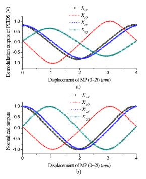
Fig.6. PCIDS signals in a single period when l/g=4: a) demodulation outputs of PCIDS as  $X_{IN}$ ,  $X_{2N}$ ,  $X_{IQ}$ ,  $X_{2Q}$ ; b) normalized waveforms as  $X'_{IN}$ ,  $X'_{2N}$ ,  $X'_{IQ}$ ,  $X'_{2Q}$ .
