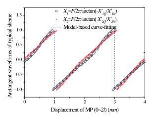
Fig.7. Arctangent waveforms directly from normalized waveforms under measurement disturbances.
