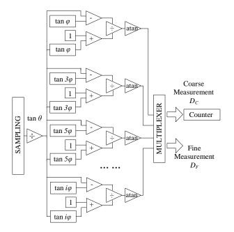
Fig.3. Principle of PSA interpolation method.
