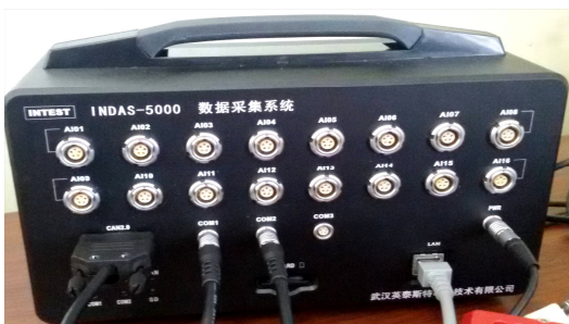
Fig.14. Data acquisition system.
