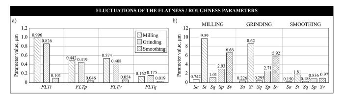
Fig.6. Fluctuations in the values of the flatness parameters (a) and group of primary and secondary surface roughness amplitude parameters (b) for selected machining processes used in experimental investigations.
