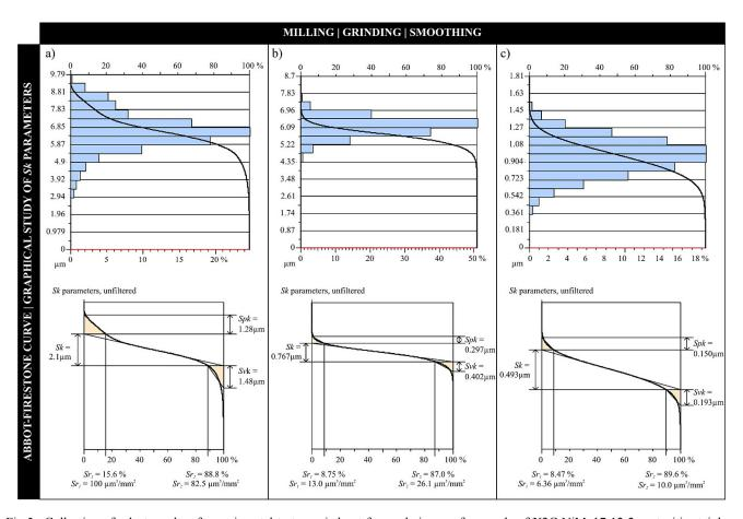
Fig.5. Collection of select results of experimental tests carried out for workpiece surface made of X2CrNiMo17-12-2 austenitic stainless steel obtained by stylus profilometer Hommel-Tester T8000 produced by Hommelwerke with HommelMap Basic 3.1.0 software in the form of an Abbott-Firerstone curve (top) and graphical studies of *Sk* parameters (bottom) after the: a) milling process, b) grinding process, c) smoothing process.
