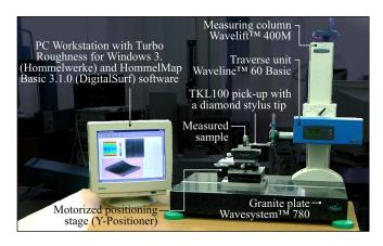
Fig.1. Stylus profilometer Hommel-Tester T8000 produced by Hommelwerke GmbH (Germany) used in the experimental tests.
