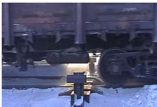
Fig.8. Laser diagnostic system COMPLEX for wheel pair inspection operating in winter conditions at the West-Siberian Railway.
