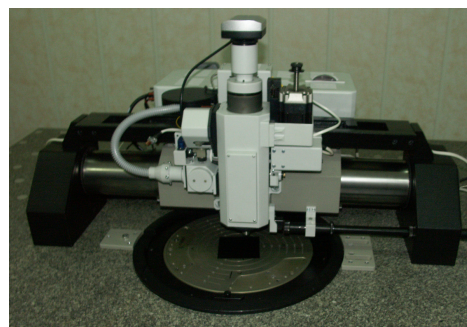
Fig. 15. The updated pattern generator using semiconductor UV laser.
