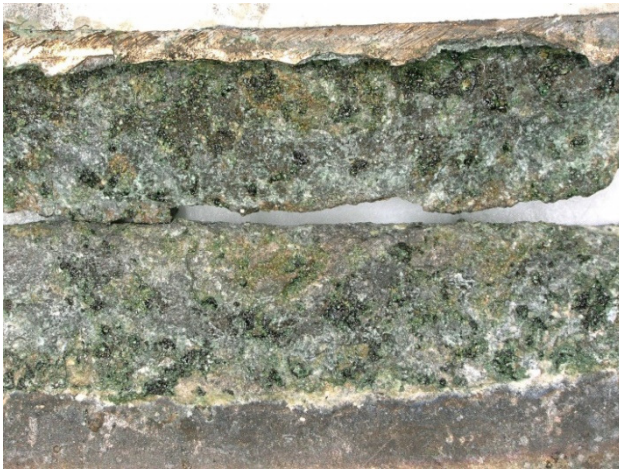
Fig. 5 Crack area after tensile test
